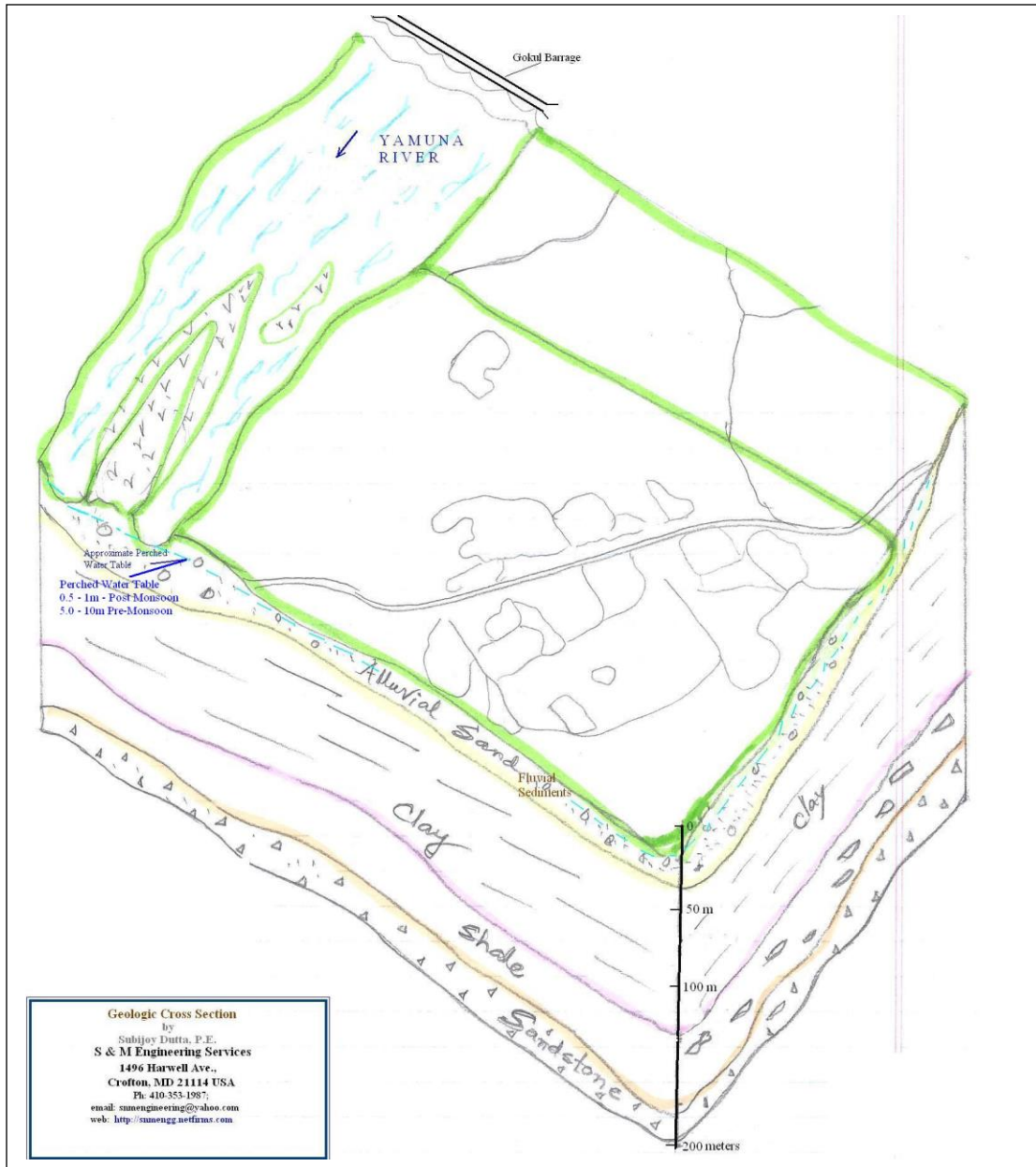
Figure 6. Typical Hydrogeologic Cross-section for the General Gokul Area
